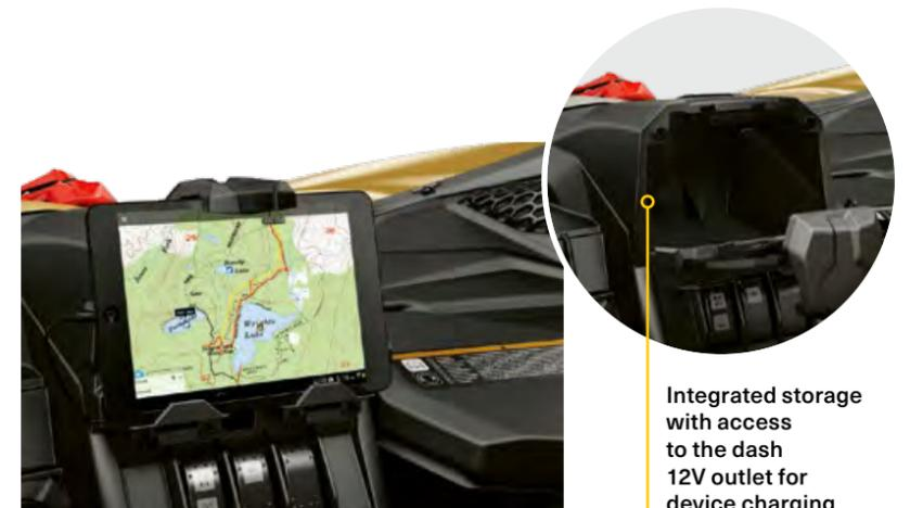
Integrated storage with access to the dash 12V outlet for device charging
