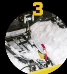
3 Lift the plow until it clips onto the mounting plate.
