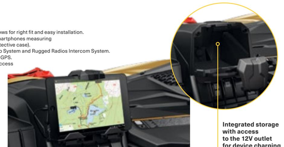
Integrated storage with access to the 12V outlet for device charging
